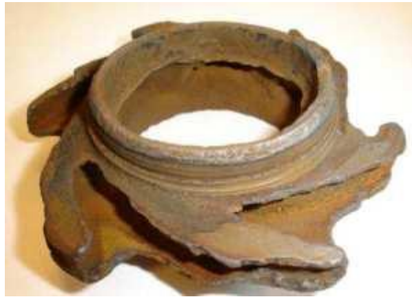
Fig. 9: Graphitic corrosion of an impeller made of grey cast iron.
