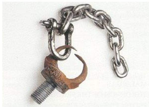
Fig. 7: Galvanic corrosion of eye bolt connected to a stainless
