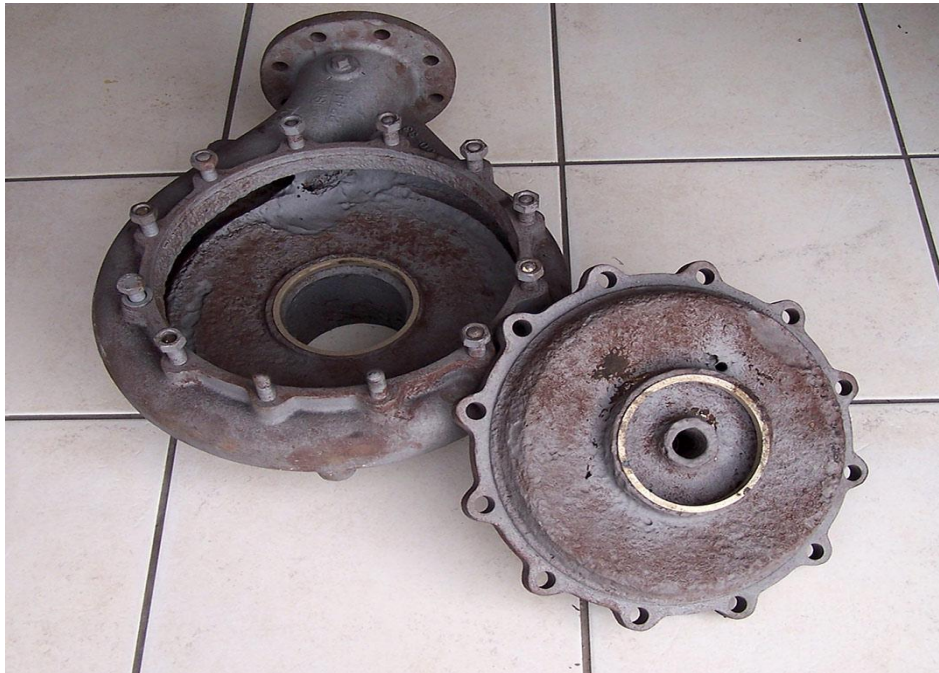
Fig. 12: Erosion damage of a pump.
