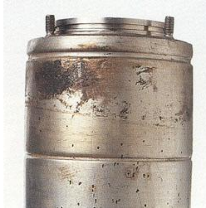
Fig. 2: Pitting corrosion on a stainless steel stator housing operating in seawater.
