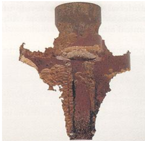
Fig. 5: Erosion-corrosion of an impeller.
