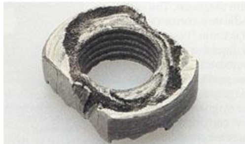
Fig. 4: Crevice corrosion on a stainless steel nut exposed to seawater.
