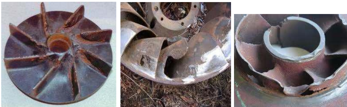
Fig. 14: Cavitation damage in some pumps. Note the tag team effect caused by erosion and corrosion
