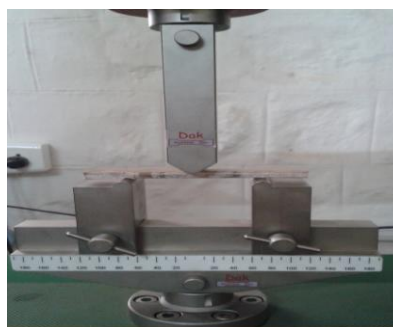
Fig. 2 Experimental testing on flexural
