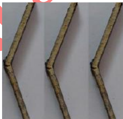
Fig . 7 Tested specimen of after flexural test carbon, sisal and rice husk
