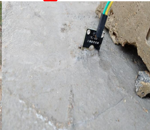
Fig. 2: Moisture sensor embedded in Concrete
