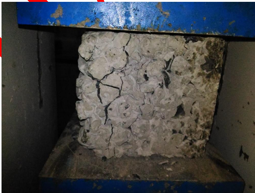
FIGURE 5:FAILURE OF CUBE COMPRESSIVE STRENGTH
