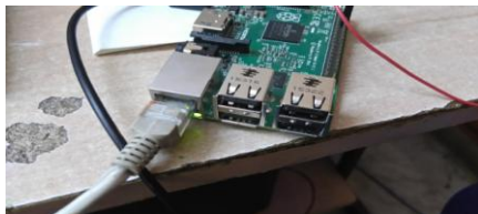
Figure 7(b): LAN connection to RPi.
