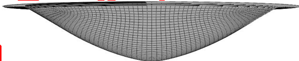
Fig. 7 Deformed sheet simulated by inward volume acceleration loading, for IF210
