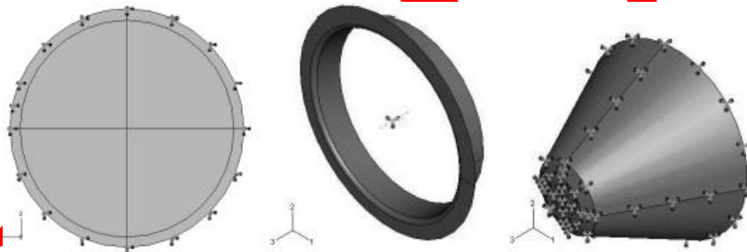
Fig. 3 Boundary conditions in EHF simulation
