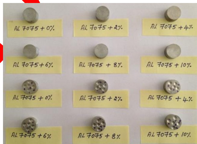
Figure 1: Hardness Test specimens before and after Indentation.
