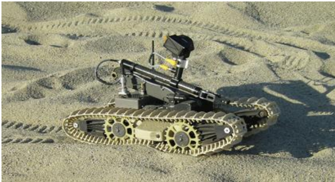
Figure 3: Small Unmanned Ground Vehicle (SUGV)
