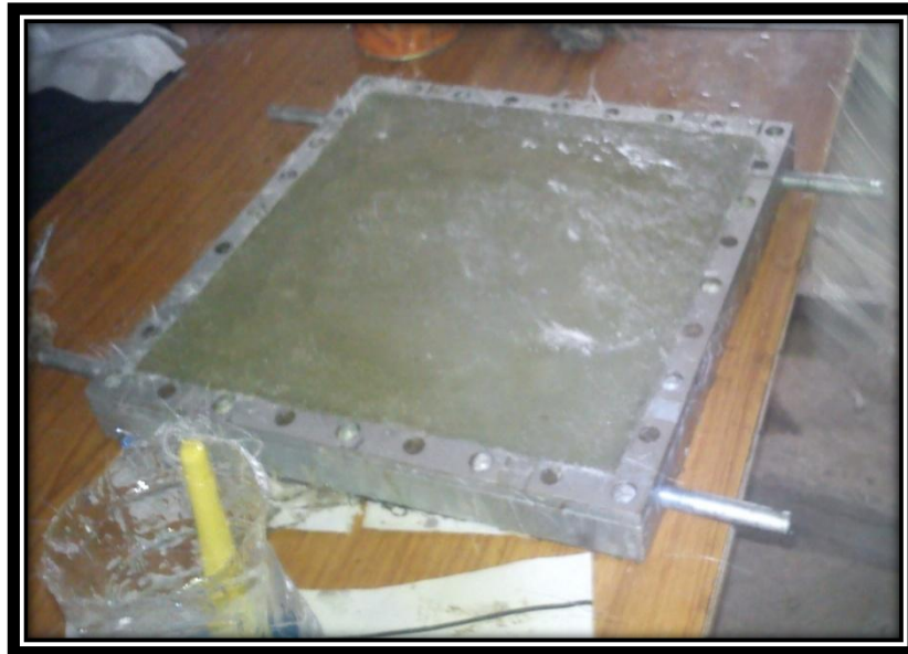
Fig.4.1, glass fiber and resin over the bottom plate of mould
