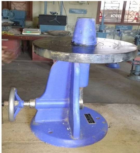
Figure 2 Flow test apparatus for cement mortar
