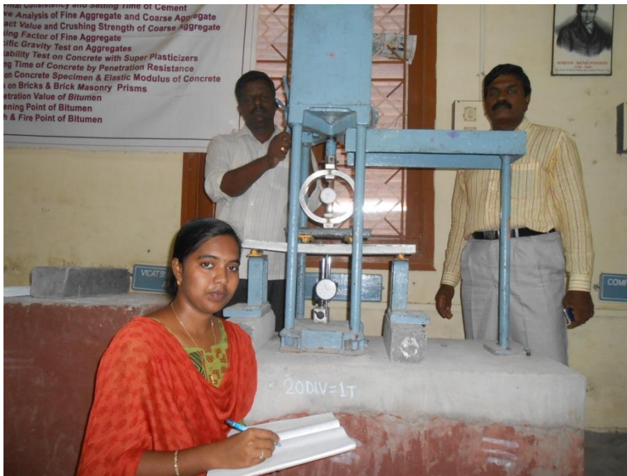
Figure 8 Actual Test set up of ferrocement panel
