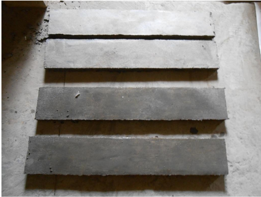
Figure 6 Prepared ferrocement panels
