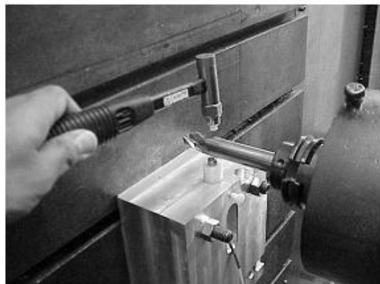
Fig 5. Rotating Tool Frf Measurement Set Up
