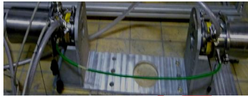
Figure 5. Optical bench Detector mounted on the left. Laser mounting on the right[15].
