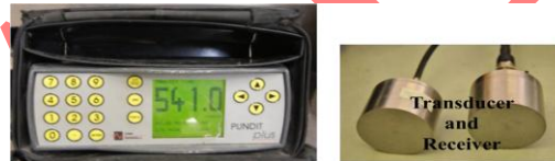
Figure 7. Ultrasonic pulse velocity test equipment (PUNDIT-PLUS) [25].
