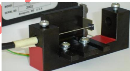
Figure 6. View of a piezo bender actuator on a test stand
