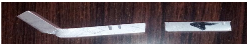
Figure 6. An impact test specimen
