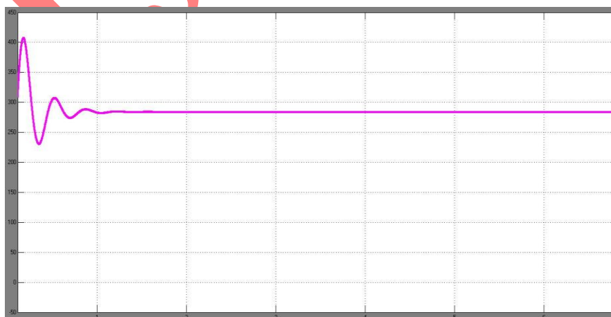
Figure 8. Closed Loop response of NARMA-L2 Controller
