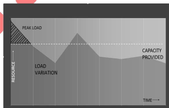
Fig. 3 Loss of traffic due to negative impact of under provisioning of resources in static resource allocation
