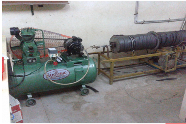
Fig. 1. Rotary drum covered with an insulation of 15mm Polyurethane foam cover
