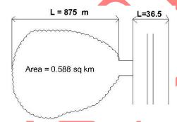
The details of the drainage and its characteristics were obtained from various reports pertaining to the area. The drainage area corresponding to this loaction is 0.588 km<sup>2</sup> and length of drainage is 875 m. The drainage area is lying in the region of Hydrological zone I. The intensity duration curve (IDF) for this zone is available as given in the following Fig-5 and hence the same is being used in the present study.
