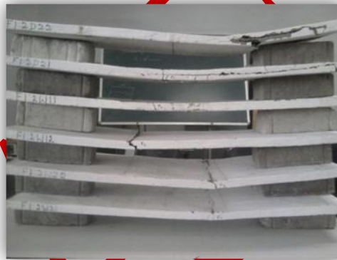
Fig 7.2 Deflected shapes of Slabs
