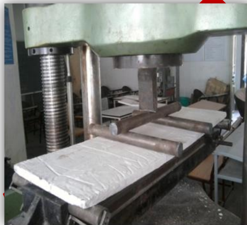
Fig 6.7 Flexural test of Ferro cement slabs
