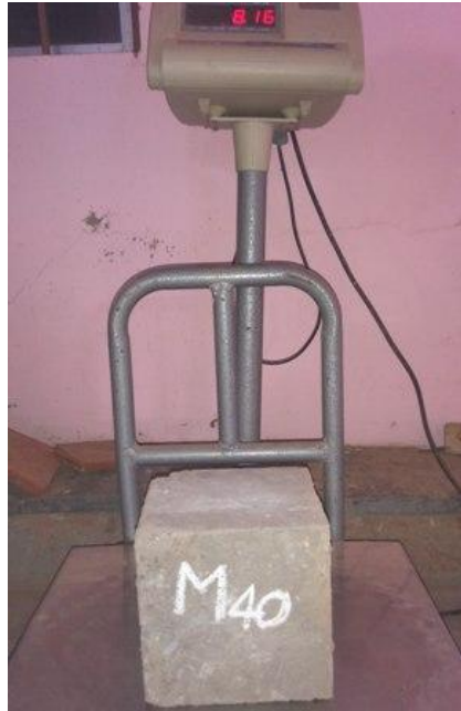
WEIGHMENT OF DRY CUBE 150X150X150MM
