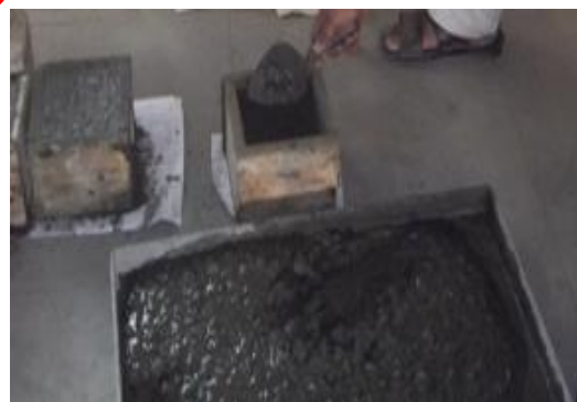
LAYING OF CONCRETE IN MOULDS
