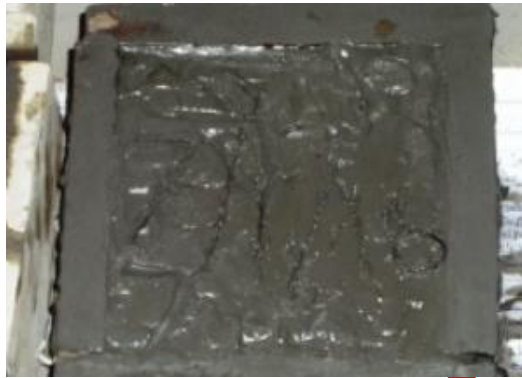
CONCRETE LAID IN MOULDS
