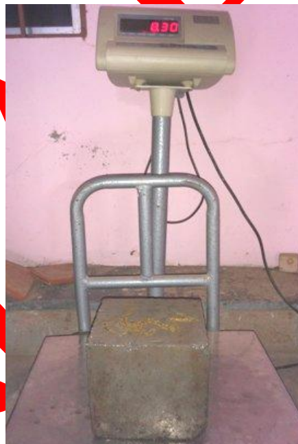
WEIGHMENT OF CUBE DIPPING IN SEAWATER FOR 40DAYS
