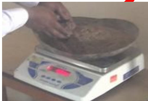
WEIGH UP OF FINE AGGREGATE
